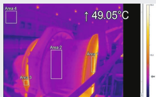
Figure 2: Mining/materials sector: thermal image of mill cylinder with four interest areas defined
